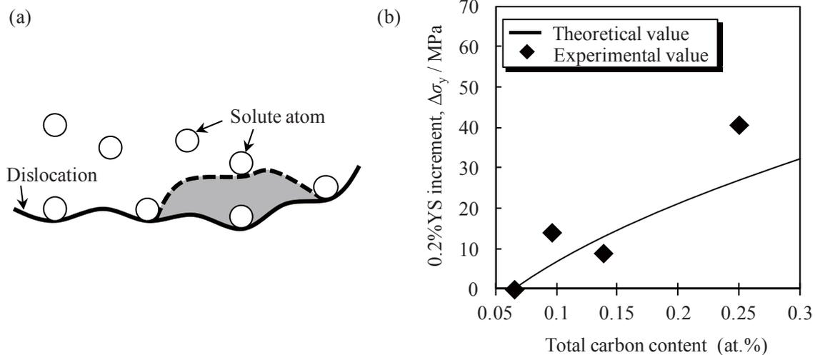
**Fig. 7** Schematic model of solid solution hardening (a) and comparison of theoretical and experimental values of 0.2%YS increment of COMP1-4 specimens (b).
