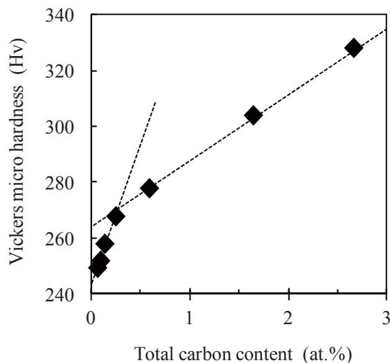
**Fig. 6** Dependence of Vickers micro hardness of COMP1-7 specimens on total carbon content.
