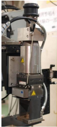
(b) Welding head
