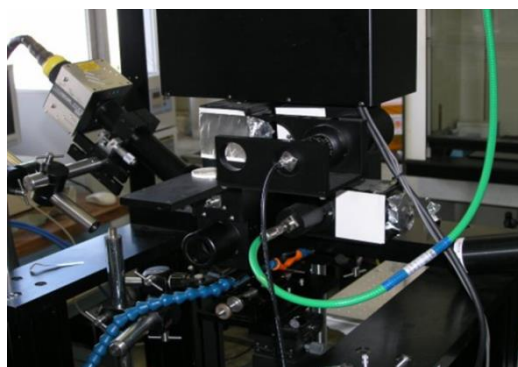
Fig. 2.7 General view of laser welding head equipped with in-process monitoring sensors.
