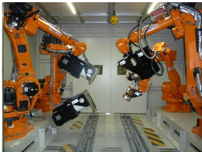
Fig. 2.14 New type X-ray transmission real-time observation system for observing keyhole and three-dimensional melt flows in molten pool.
