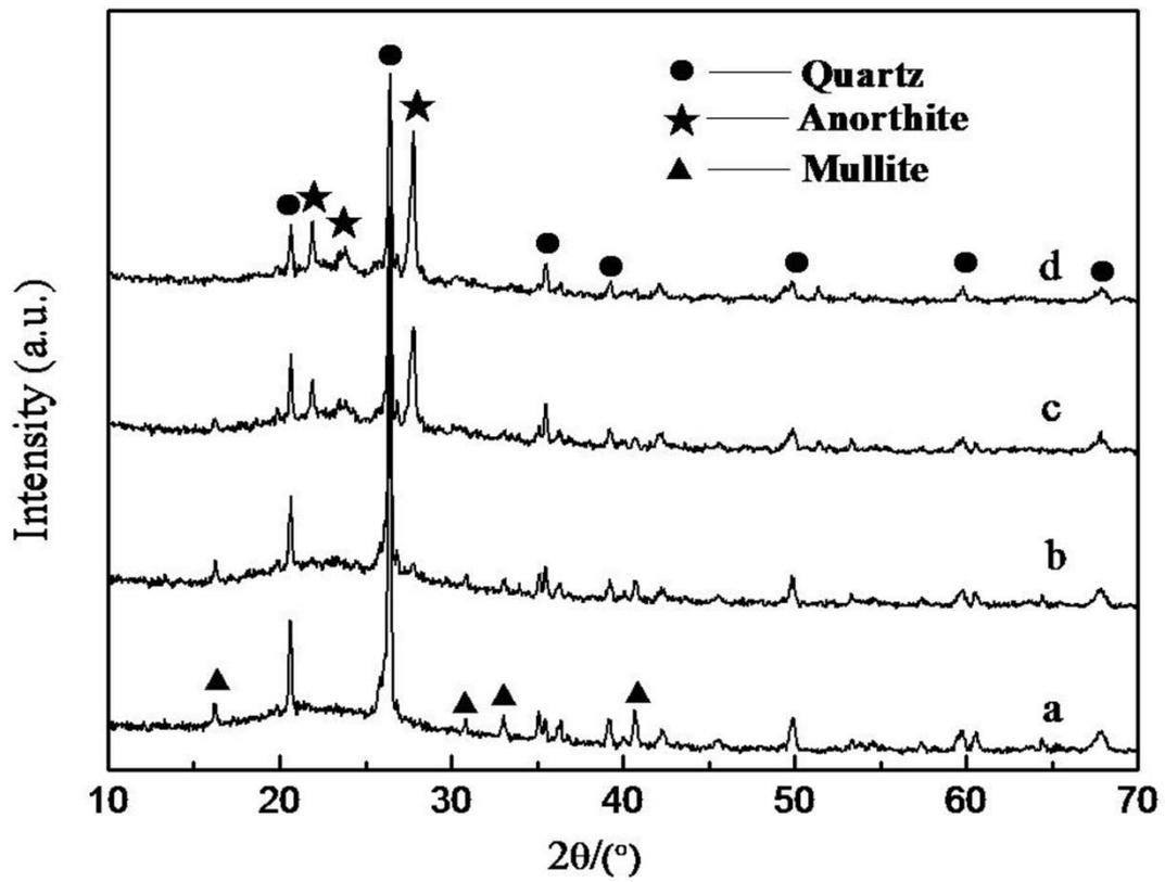
Fig. 3.8 XRD data for porcelain with (a) 0 mass%, (b) 2 mass%, (c) 4 mass%, and (d) 6 mass% CaO addition.
