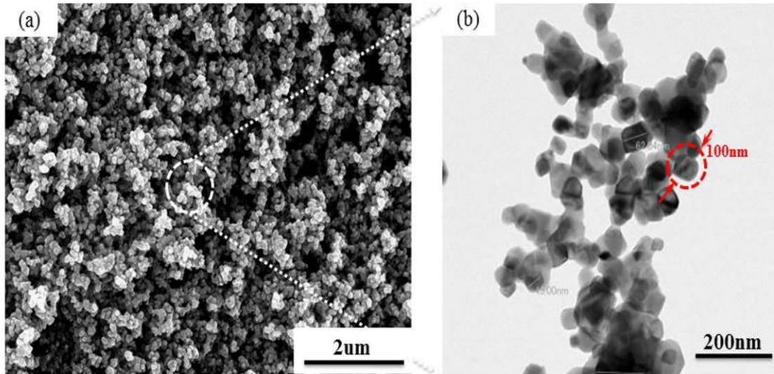
Fig. 4.4 SEM and TEM images of the synthesized NiO-YSZ composite powder (sample-2) calcined at 1000°C. (a) SEM image; (b) TEM image.
