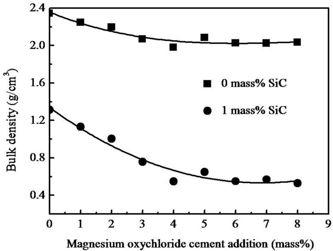
Fig. 2.5 Effect of MOC content on the bulk density of fired porcelain bodies without and with 1 mass % SiC at 1200°C.
