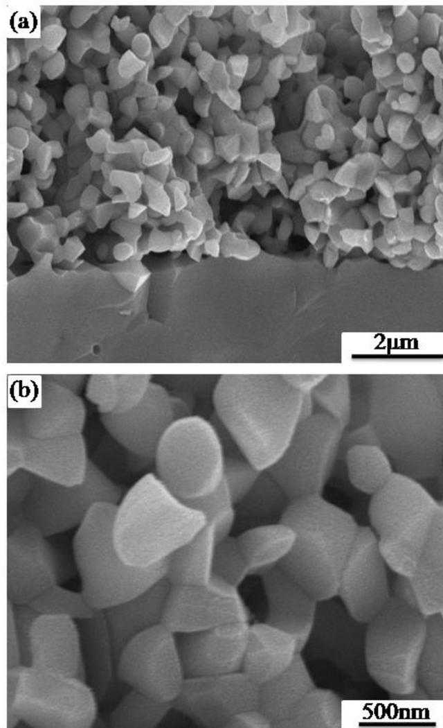
Fig. 4.8 SEM images of the Ni/YSZ anode after electrochemical performance testing
