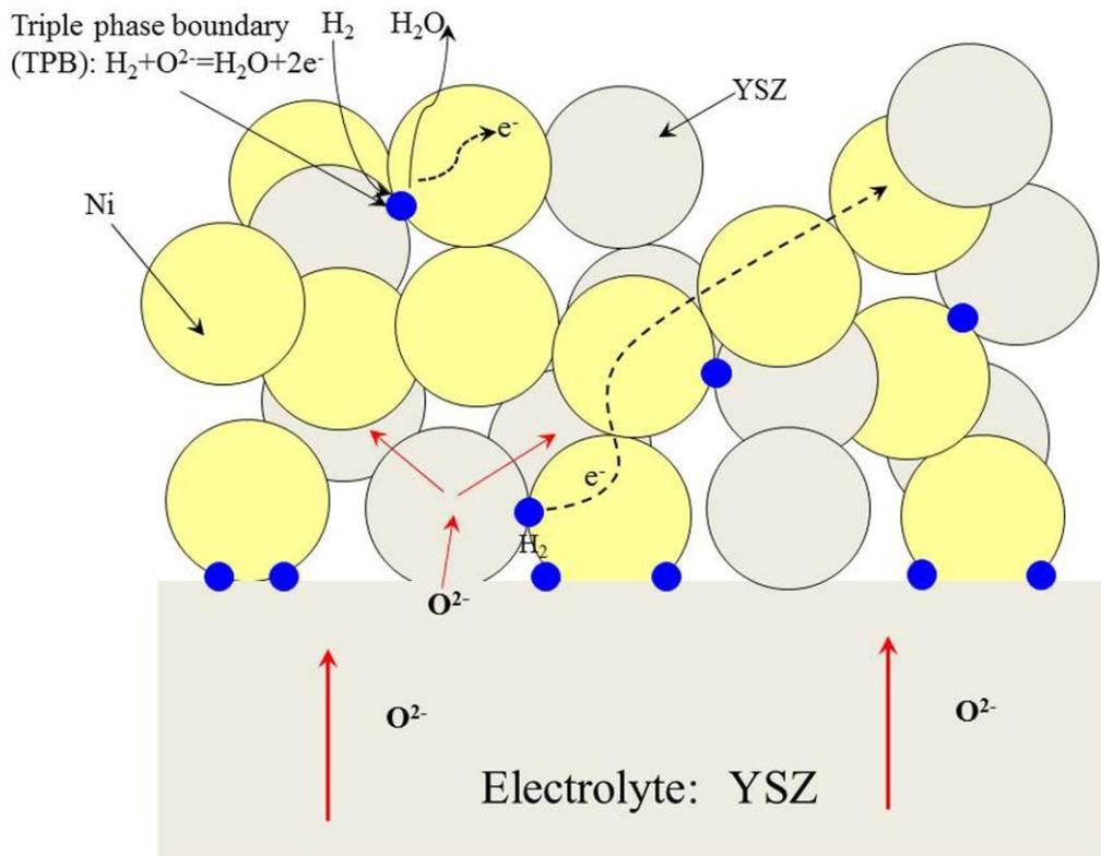
Fig. 1.3 Schematic illustrations of Ni-YSZ anode structure.
