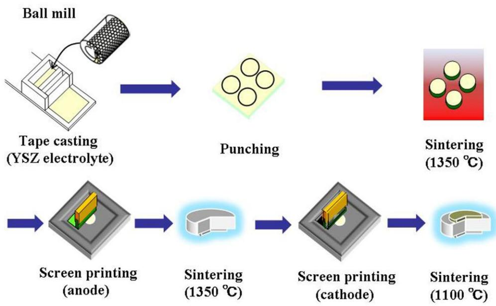
Fig. 4.2 Flow chart of the cell fabrication.
