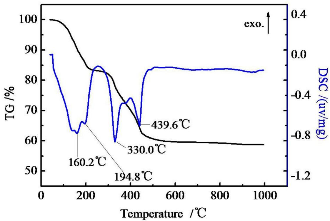
Fig. 2.6 TG-DSC curve of the MOC powder.
