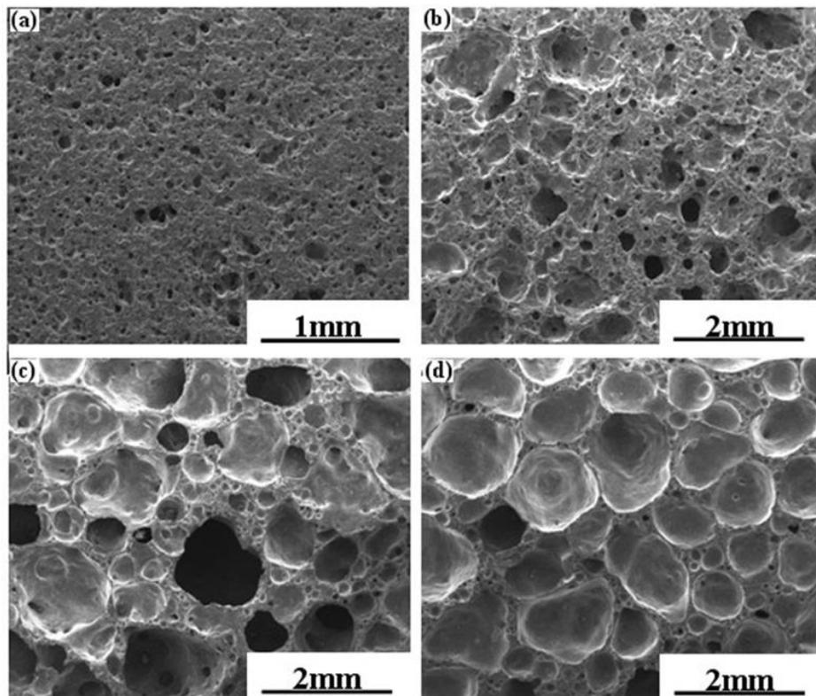
Fig. 2.9 SEM micrographs of the fired porcelain bodies with 1 mass% SiC:
