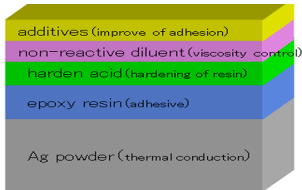
Fig.1.3 Composition of Ag filled epoxy
