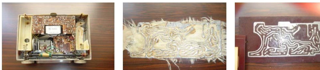
Fig.1.2 Photo of electro devices using ICA. (a) Terminal attached with electro conductive adhesive, (b) Circuit by the conductive adhesive on glass crossing, and (c) Conductive adhesive circuit on a Bakelite substrate (Photo:JPCA)
