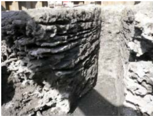
Fig. 4.7 Cross section of JETCRETE by the nozzle with flow conditioner
