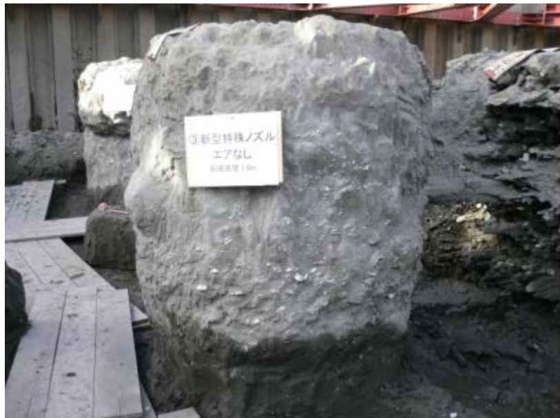
Fig. 4.22 Type 3 : JETCRETE column by the nozzle with flow conditioner without air
