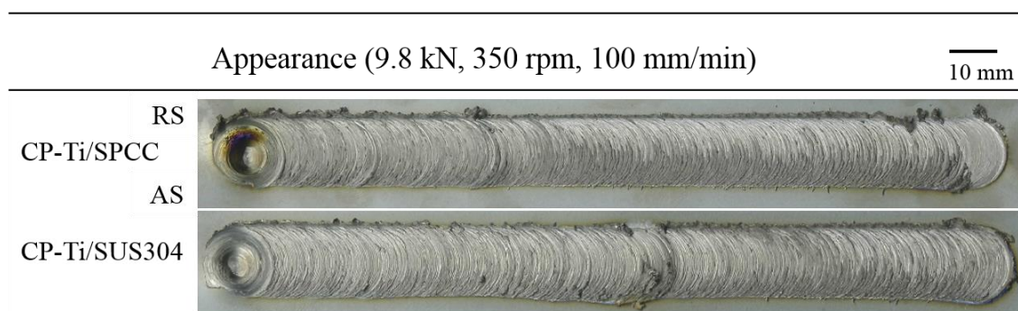
Fig. 3.4 Appearances of the lap joints of CP-Ti/SPCC and SUS304 with 350 rpm and 100 mm/min.
