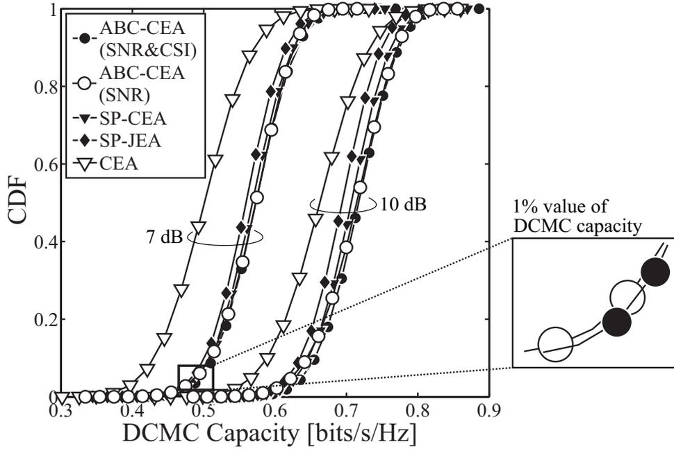
Figure 4.9: DCMC capacity performance in balanced SNR.
