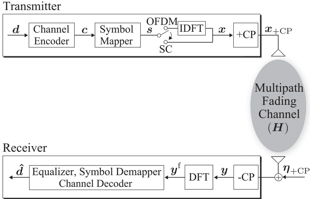
Figure 2.7: Block diagram for a broadband wireless transmission.
