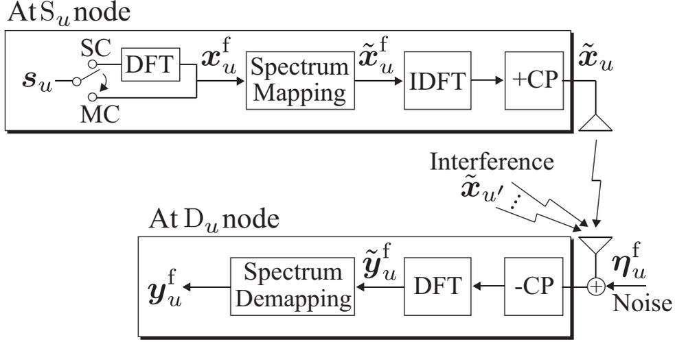
Figure 3.1: Signal model of DSC for  $S_u$ - $D_u$  link.
