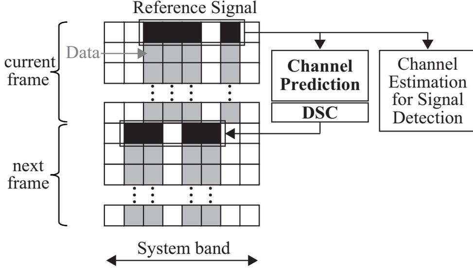
Figure 3.2: Reference signal spectrum placement for channel prediction.
