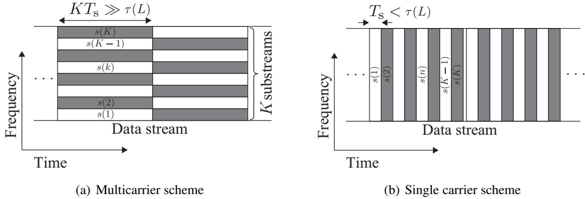
Figure 2.5: The concept of broadband transmission schemes.
