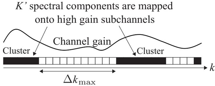
Figure 3.5: Cluster-featured transmission band in DSC.
