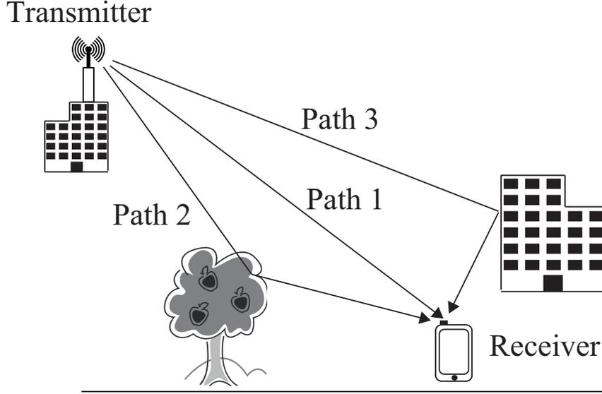
Figure 2.1: Illustration of the physical multipath environment.
