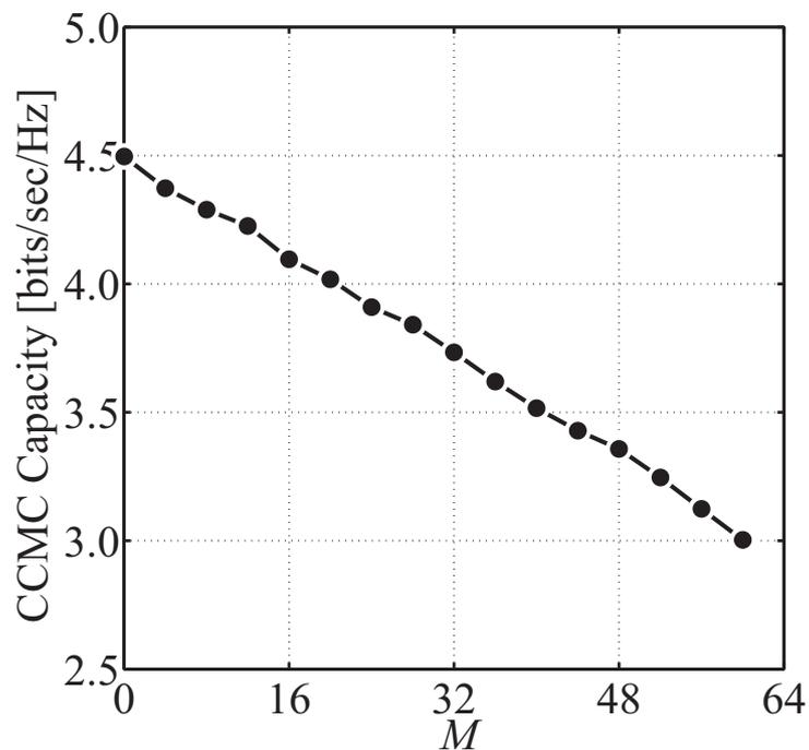
Figure 3.9: CCMC capacity for the present frame when  $M$  varies.
