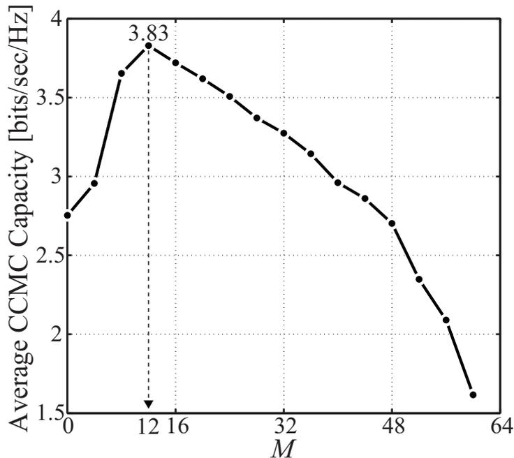
Figure 3.8: Average channel capacity when  $M$  varies.
