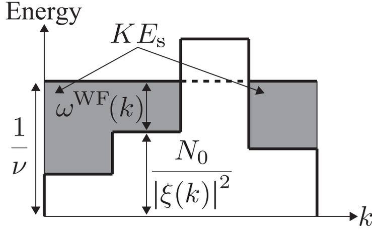
Figure 2.10: An illustration of water-filling principle based transmit spectrum optimization.
