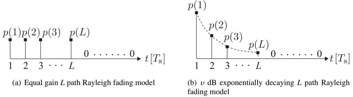
Figure 2.4: Delay power profiles of two widely used channel models.
