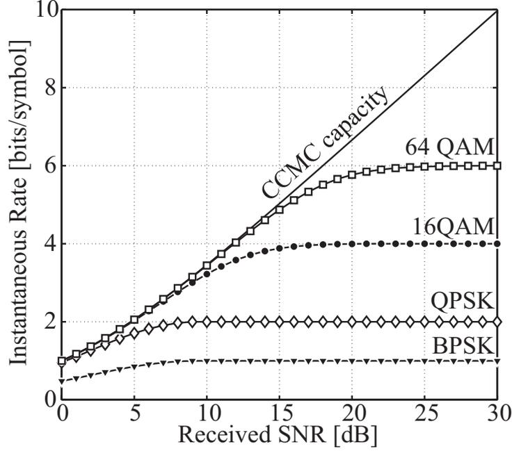
Figure 2.9: Maximum achievable rates for discrete modulation schemes in AWGN channel.
