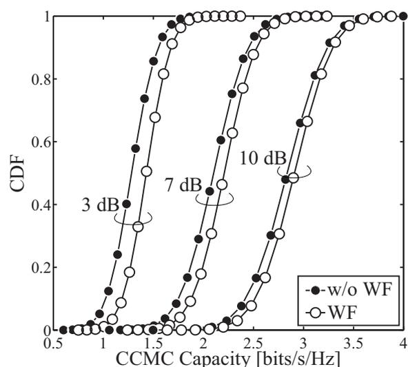
Figure 2.11: CCMC capacity of water-filling principle.
