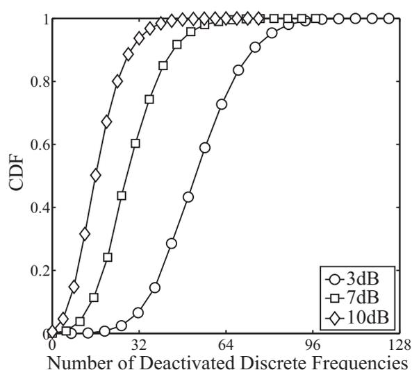
Figure 2.12: Number of subchannels deactivated by water-filling principle.
