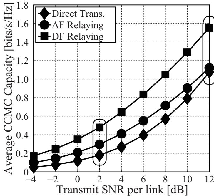
Figure 2.22: CCMC capacity comparison between relaying schemes and direct transmission.
