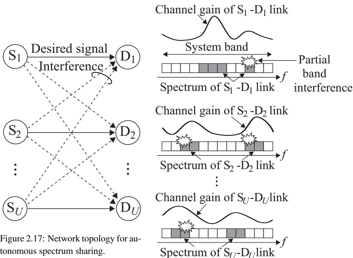
Figure 2.17: Network topology for autonomous spectrum sharing.
