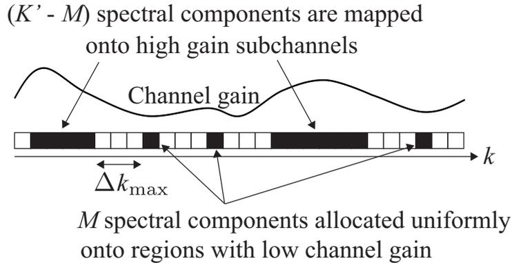
Figure 3.7: Channel prediction reliability guaranteeing subchannel selection.
