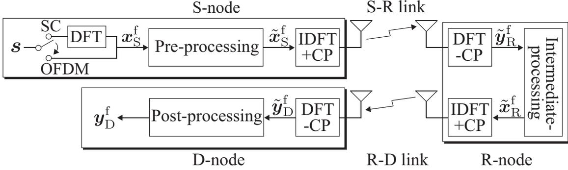
Figure 4.1: Schematic of two-hop AF broadband relaying.
