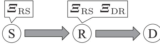
Figure 4.2: Assumption of availability of CSI in the considered two-hop broadband relaying.
