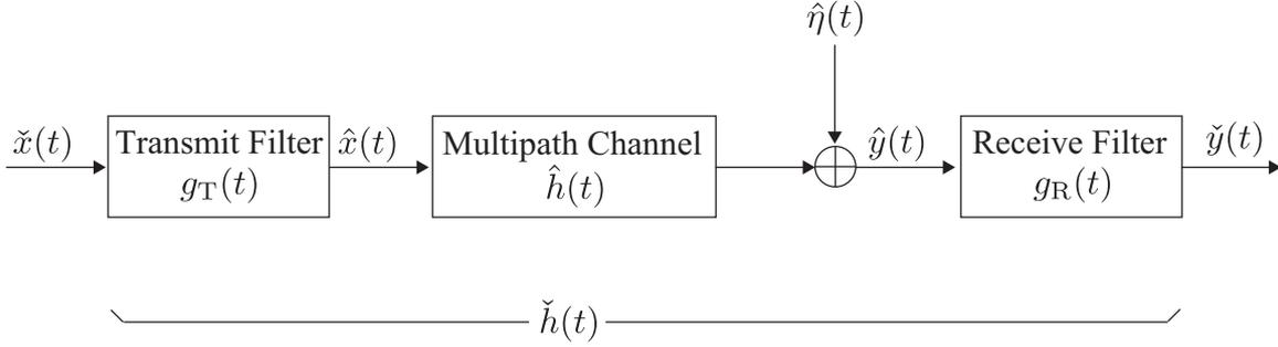
Figure 2.2: Baseband transceiver for transmission over multipath channel.
