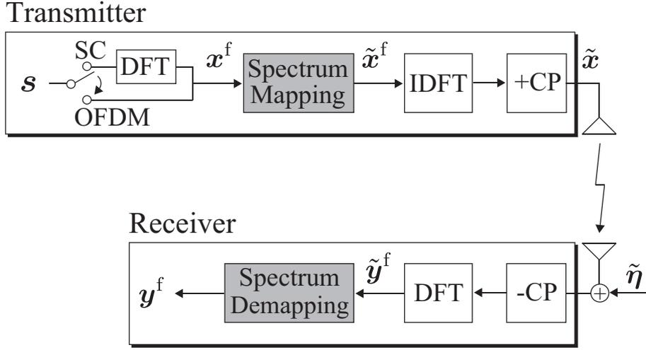
Figure 2.13: Simplified signal model to realize BAR Control.
