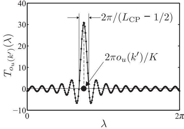
Figure 3.3:  $T_{o_u(k')}(lambda)$  when  $K = 256$ ,  $o_u(k') = 83$  and  $L_{CP} = 16$ .
