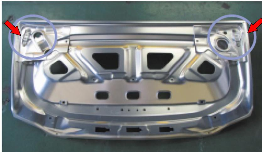
**Fig.1-9** An example of Al-alloy/Steel FSSW application (trunk lid parts) <sup>27)</sup> .
