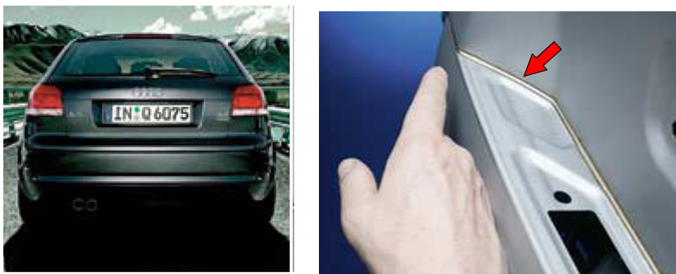
Fig.1-5 An example of the steel trunk-lid by Laser brazing method (diode-laser) 33) .
