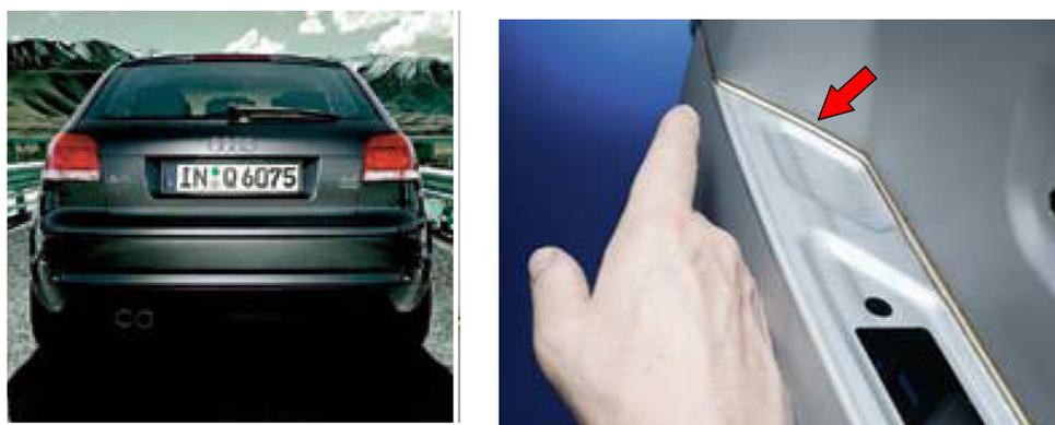
**Fig.1-5** An example of the steel trunk-lid by Laser brazing method (diode-laser) <sup>33)</sup>.
