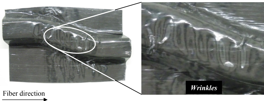
Fig.5.9 Appearance of wrinkling in forming process
