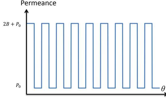
Fig. A1.5 Permeance in the air gap.
