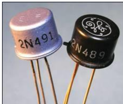
Figure 1. The unijunction transistor developed at GE in the early 1950s [2].
