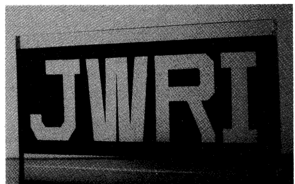
Fig. 50 Ceramic-plastic composite produced by ceramic thermal spraying.
