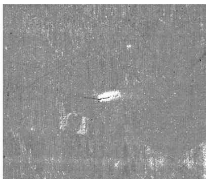
Fig. 6-2 An example of a crack initiated on Type 316L stainless steel.
