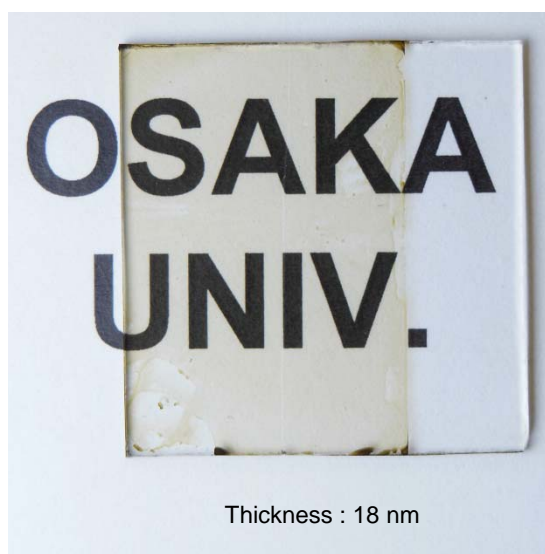
Figure 4. Photo of the spin-coating film formed with the aqueous 2% (w/w) solution of the pyridinium salt of PMAP (molar ratio = 1:2 based on the aniline unit) on a glass substrate (26 x 26 mm) and its thickness.
