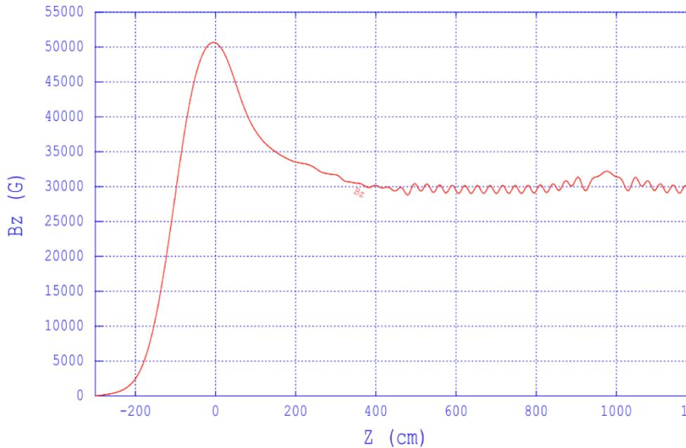
Figure 2.5: Magnetic field distribution along the COMET beam line.
