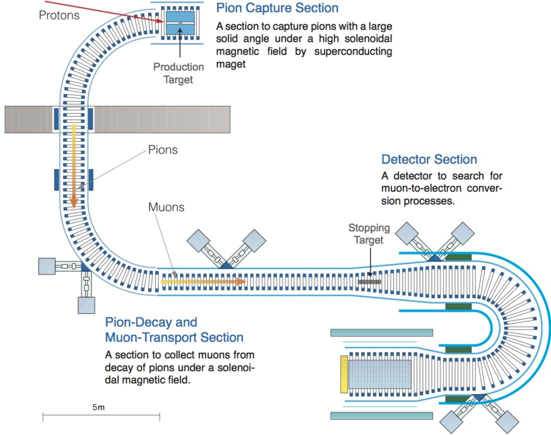
Figure 2.6: Schematic layout of the COMET beam line.
