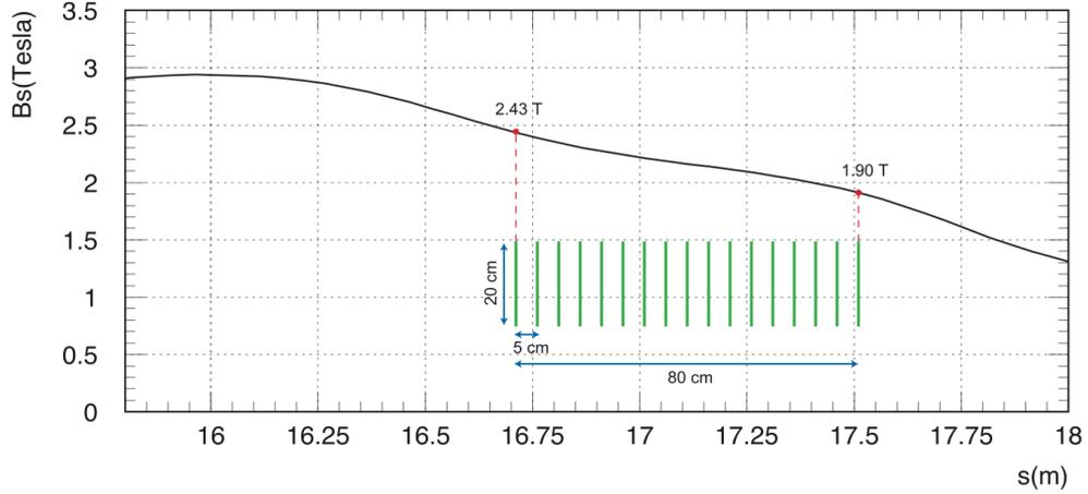
Figure 2.8: The graded magnetic field near the stopping target region.
