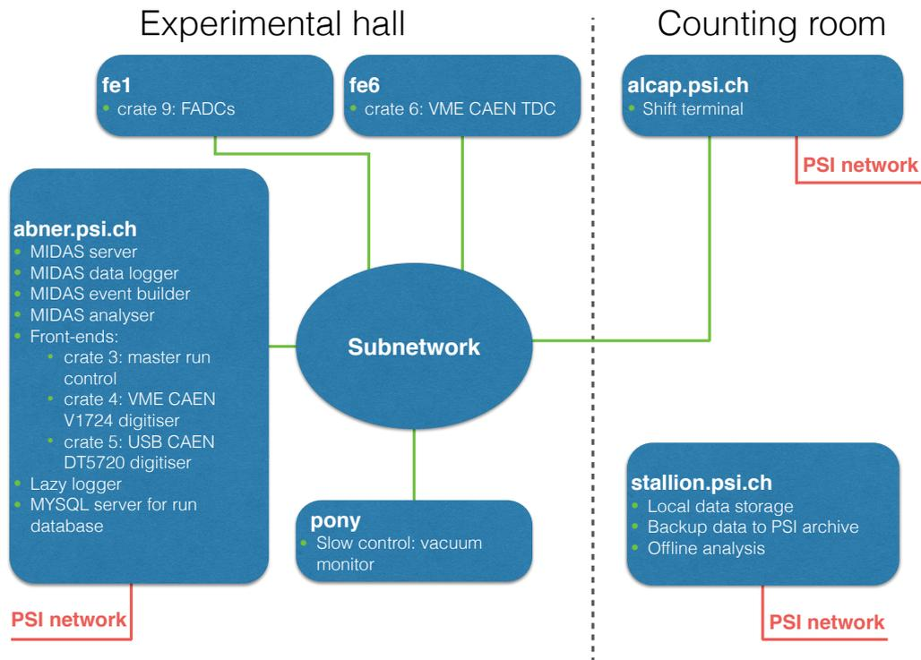
Figure 4.7: AICapDAQ in the Run 2013. The fe6 front-end is a VME single board computer belongs to the MuSun group, reads out the upstream detectors.
