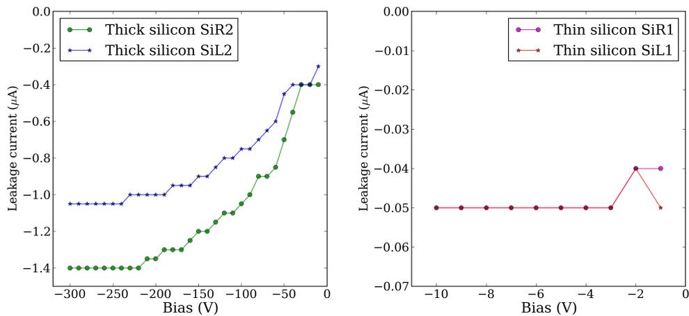
Figure 4.4: Leakage currents of the silicon detectors under bias.
