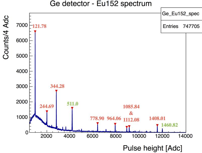
Figure 4.9: Energy spectrum of the  $^{152}\text{Eu}$  calibration source recorded by the germanium detector. The most prominent peaks of  $^{152}\text{Eu}$  along with their energies are annotated in red; the 1460.82 keV line is background from  $^{40}\text{K}$ ; and the annihilation 511.0 keV photons come both from the source and the surrounding environment.
