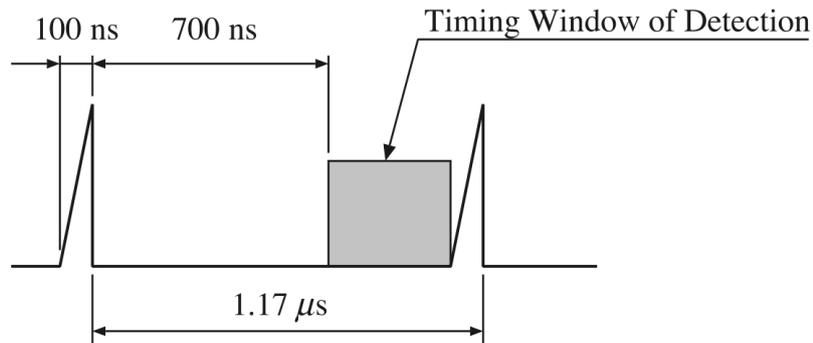
Figure 2.10: Timing window of detection.
