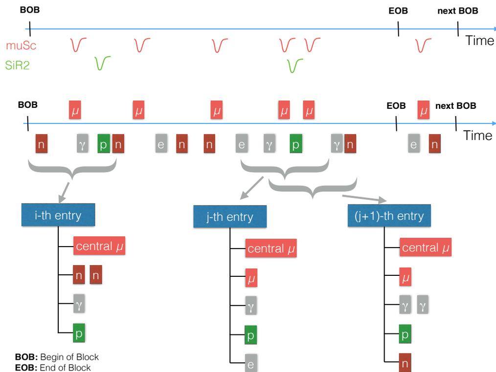
Figure 4.13: Concept of the AICap analysis code: pulses from individual detector in blocks of time are analysed, then sorted centred around stopped muons.
