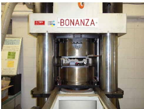
Figure 6.3: The high pressure synthesis machine (Left) and the assembled parts on the anvils (Right).
