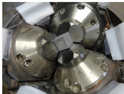
Figure 6.3: The high pressure synthesis machine (Left) and the assembled parts on the anvils (Right).
