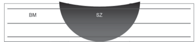
Fig.2 Schematic drawing showing the location of micro-hardness measurements
