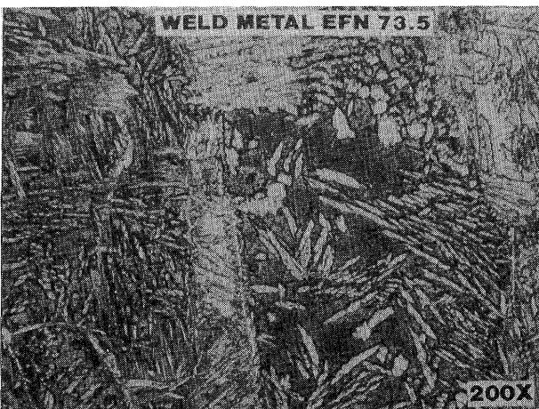
Fig. 17 Microstructure of Ferralium 255 SMA Weld Metal, FN 73.5, 200 X, Kallings Reagent.
