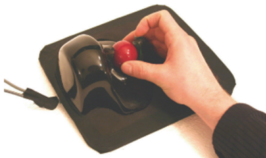
Figure 2.1: The Globefish [17]. An integral 6-DOF desktop controller.
