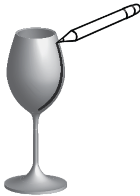
Figure 5.10: Drawing near the edges of a mesh could lead to false positives and switch the system to rotation mode.
