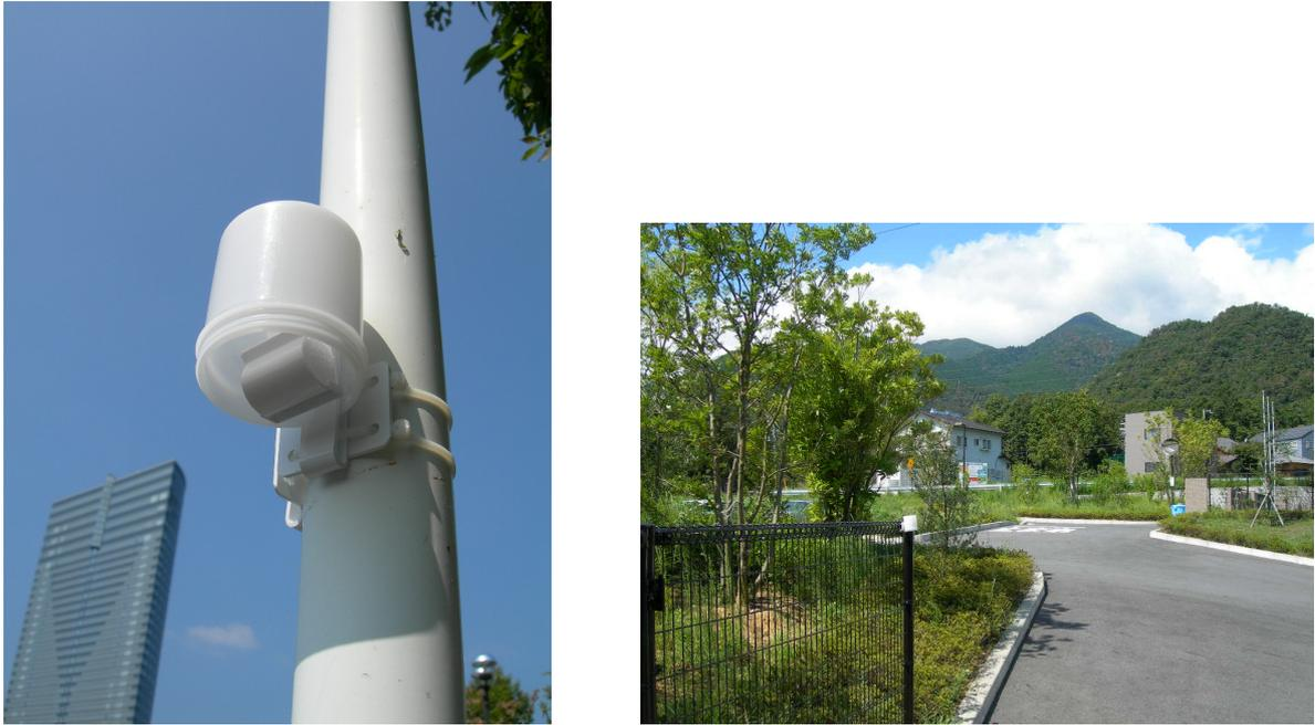
Fig. 2.4 Passive samplers during sampling.
