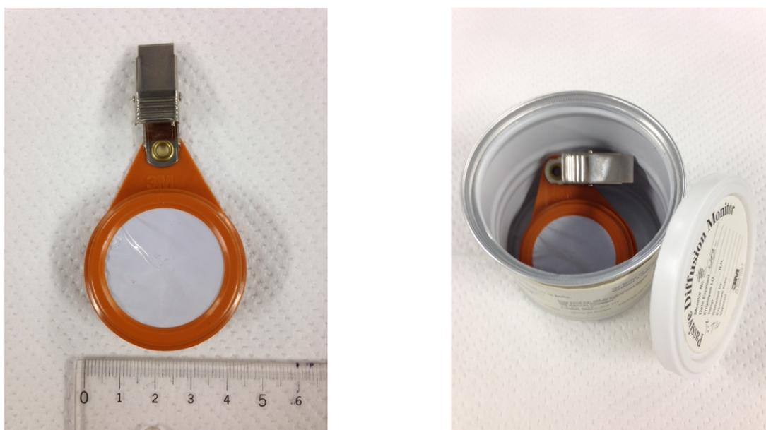
Fig. 2.3 The passive sampler for VOCs used in this study.
