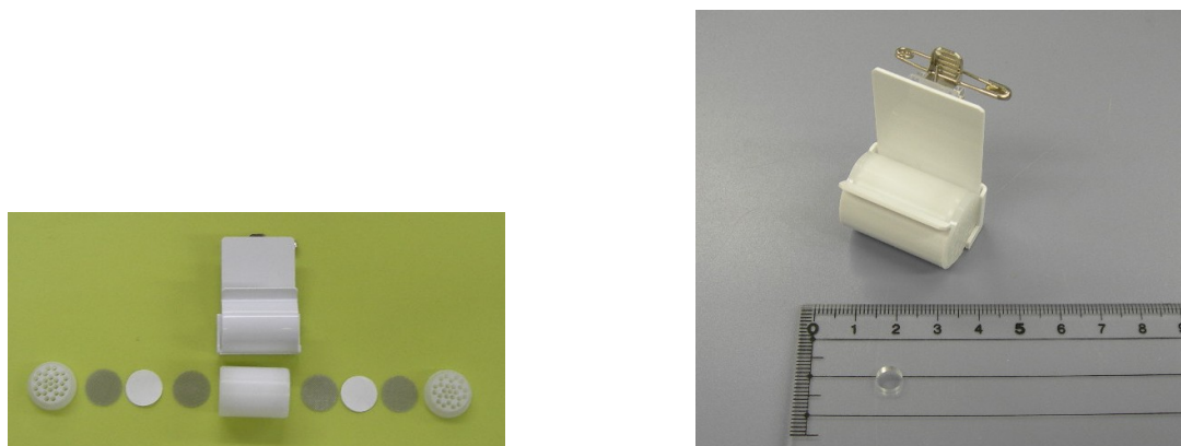
Fig. 2.2 The passive sampler for O_3 , NO_2 and NO_x used in this study.
