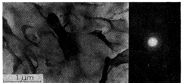
Fig. 18 Specimen 14-3: TEM micrograph of Cr 7 C 3 carbide situated at the first layer grain boundary (CER).
