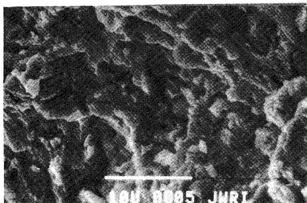
Fig. 27 SEM fractograph of the centre of 14-1 specimen overlay.
