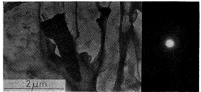
Fig. 20 Specimen 14-3: TEM micrograph of TiB boride situated at third layer grain boundary (CER).
