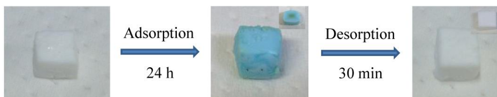
Fig. 5-6 Photographs of the blend monoliths in the processes of adsorption and desorption of \text{Cu}^{2+} (inner pictures: inside blend monolith).
