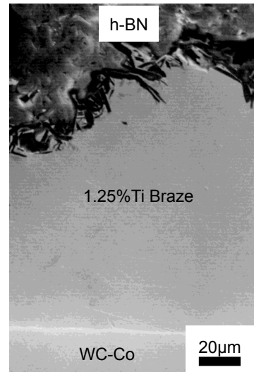
Fig. 2.10 Cross section of h-BN / 1.25%Ti braze / WC-Co interface (enlargement).
