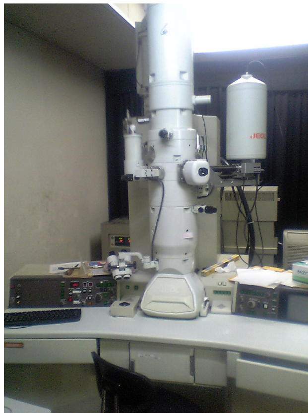
Fig. 5.2 Appearance of the Transmission Electron Microscope used in this work (JEOL JEM-2010).
