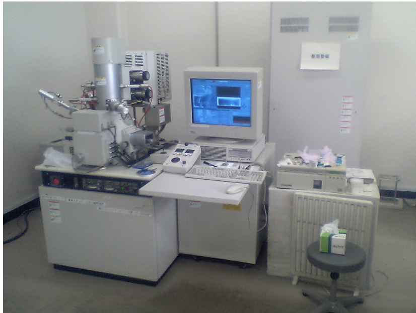
Fig. 5.1 Appearance of the focused ion beam (FIB) system used in this work.
