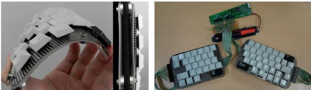
Figure 58 Second keyboard prototype showing the flexed board and the split, wireless configuration.
