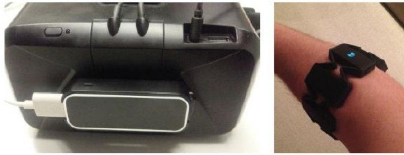
Figure 62 Oculus Rift with attached LEAP Motion for hand interactions such as button presses (left) and the arm-worn Myo to facilitate walking via natural arm movements (right).
