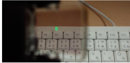
Figure 26 Image through the AiRScouter showing the virtual text and keyboard.
