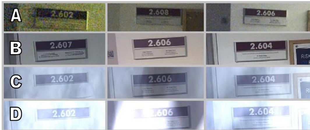
Figure 54 Door plates in various conditions. Row A is in dim emergency lighting. Row B is in standard hallway lighting. Row C is in smoke, and Row D is in heavy smoke. Note that camera exposure automatically adjusted for lighting conditions.
