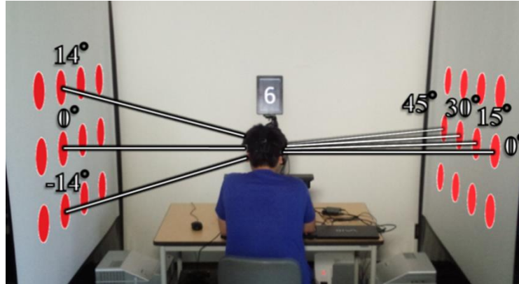
Figure 34 Experiment setup showing projector screens, numbers displayed on the tablet for the concentration task, and a participant. A simulated view of display angles and large icons at every position is overlaid for reference.
