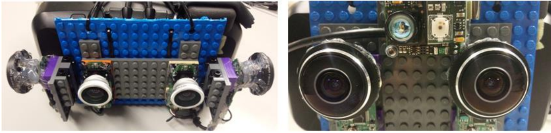
Figure 40 Side-mounted fisheye camera system for viewing peripheral and rear scene information (left), and a setup with wide-angle lenses and time-of-flight camera for hand tracking and real time 3D reconstruction (right).
