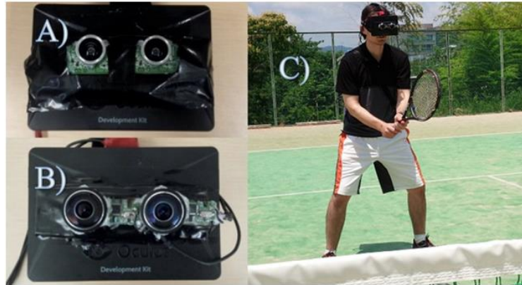
Figure 32 The A) first and B) second prototypes of the Fisheye Vision display with 180 degree and 238 degree FOV lenses, and C) testing of the 238 degree prototype in a tennis rally.
