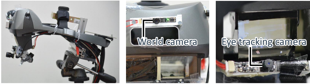
Figure 3.6: An OST-HMD equipped with an eye-tracking camera.
