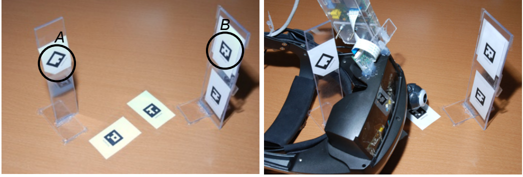
Figure 3.5: Setup for spatial calibration of the HMD. (left) The markers are arranged so that images taken by the camera can detect markers in different planes. (right) When the HMD is placed between the markers the cameras can detect the markers in the environment. We use the same device as was used by Itoh and Klinker (2014a) .
