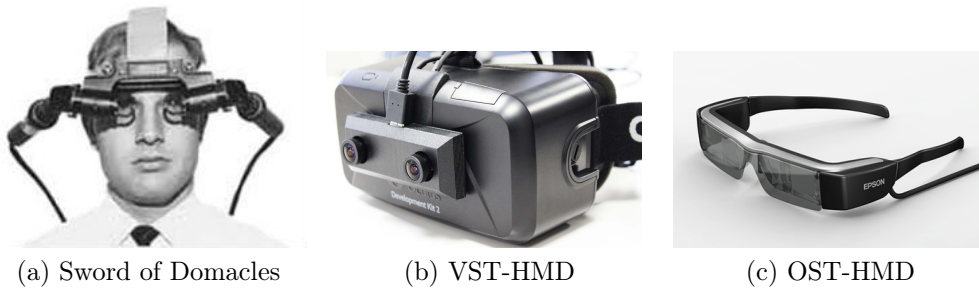
Figure 1.1: Different HMDs developed over the years. (a) The sword of Domacles — the first HMD (Sutherland (1968)), (b) Oculus Rift DK2 equipped with the Ovrvision Module — a typical VST-HMD (Oculus Rift (2015); Ovrvision (2015)), and Epson Moverio BT 200 — an OST-HMD (Epson (2015)).
