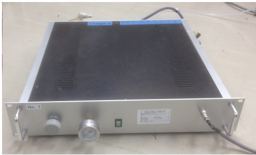
Fig. B.4: Custom-made air-pressure control device.
