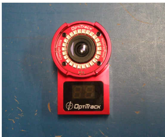
Fig. A.4: IR camera of motion capture system (Flex 3, Natural Point, Inc.)
