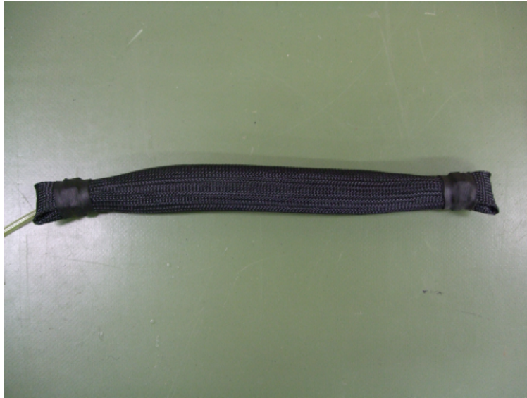
Fig. B.1: McKibben type pneumatic artificial muscles Air muscle( Kanda-tsushin Kogyo)
