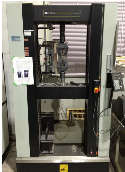
Fig. 2.11 General view of tensile test machine used.
