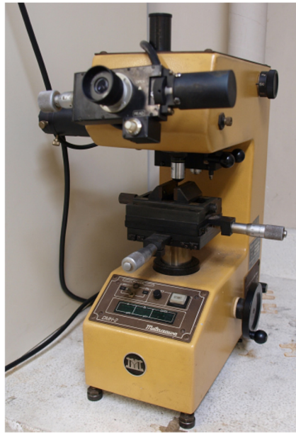
Fig. 2.10 General view of micro Vickers hardness testing machine used.
