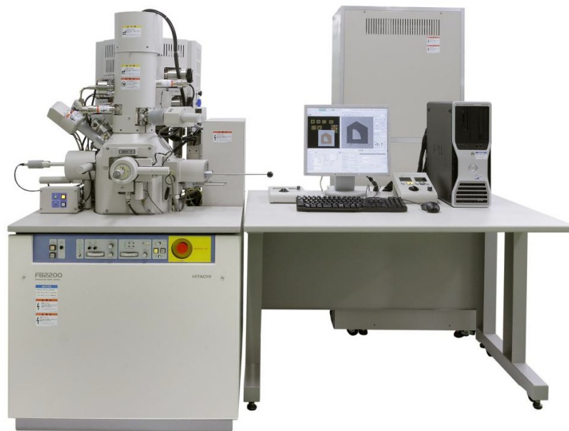
Figure 5.1 Optical image of FB2200 (Hitachi) FIB system
