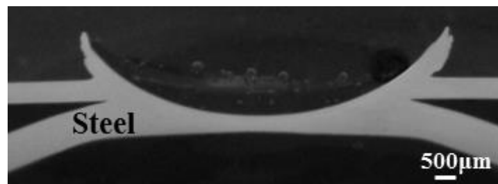
Fig.4-12 Cross-sectional macro image of the specimen after the cross tensile test (Pd: 2.2 mm).
