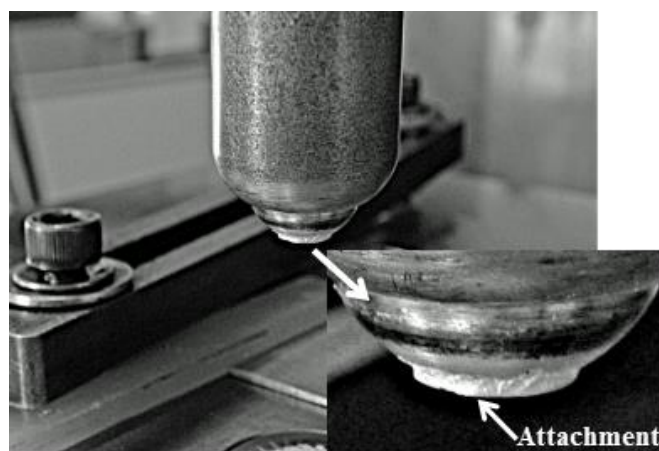
Fig.5-5 Appearance of the tip of the tool after welding of A5052 and GI steel.
