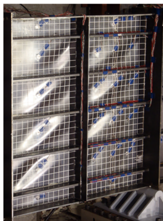
Fig. B.1 Stiffened panel specimen after shear buckling
