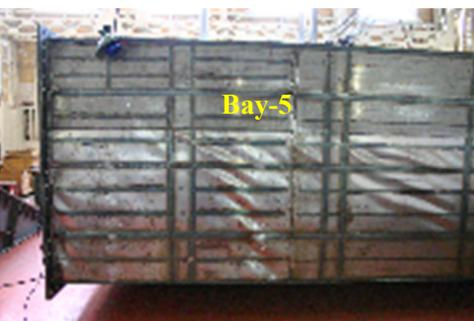
(e) Collapse of Hold-2 side shell
