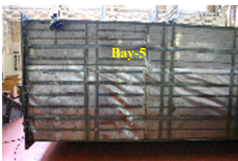
(e) Collapse of Hold-2 side shell
