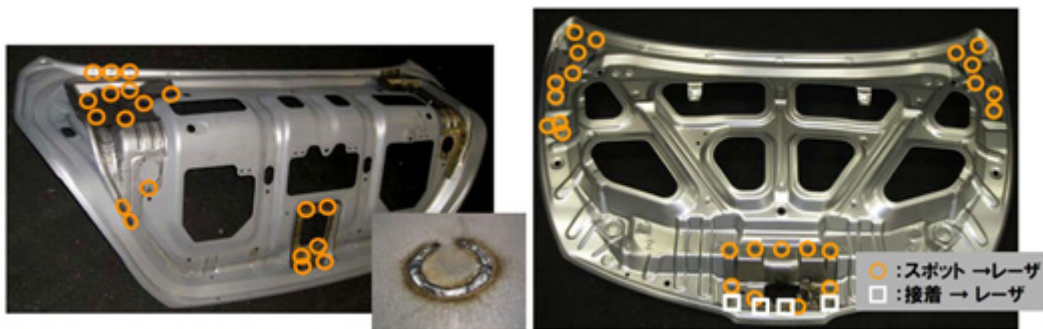
Fig. 1.16 Remote welds of TRUNK LID INR (Left) and HOOD INR (Right) 21) .
