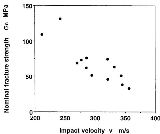
**Fig. 3** Nominal fracture strength plotted against impact velocity.
