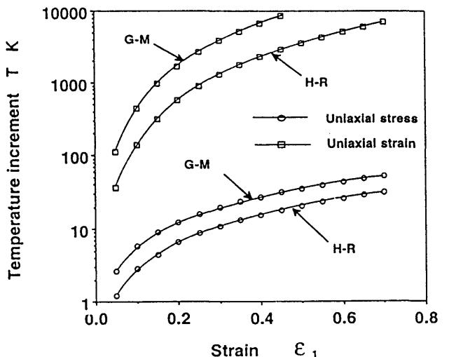
Fig. 7 Variation of numerical temperature increment against strain. G-M and H-R indicate the results obtained by strain-rate dependent and independent constitutive relations, respectively.
