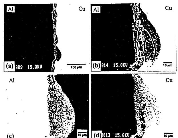
**Fig. 6** Microstrucuture (a,b) and X-ray image analyses of Al(c) and Cu(d) of Al/Cu joint welded at 333 m/s.
