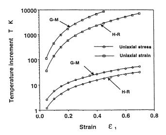
**Fig.** 7 Variation of numerical temperature increment against strain. G-M and H-R indicate the results obtained by strain-rate dependent and independent constitutive relations, respectively.
