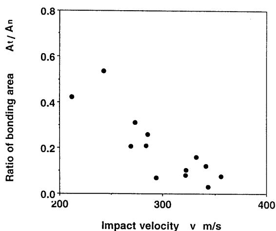
**Fig. 4** Ratio of bonding area plotted against impact velocity.
