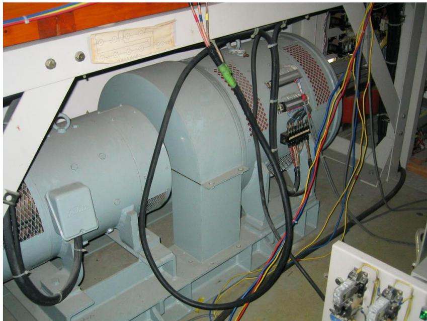
Fig. 3.25 Photo of synchronous generator moved by a dc motor.
