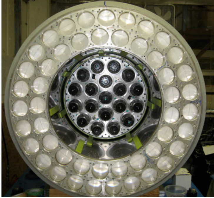
Figure 3.15: Picture of whole calorimeter consisted by NaI and 97 CsI crystals [3].
