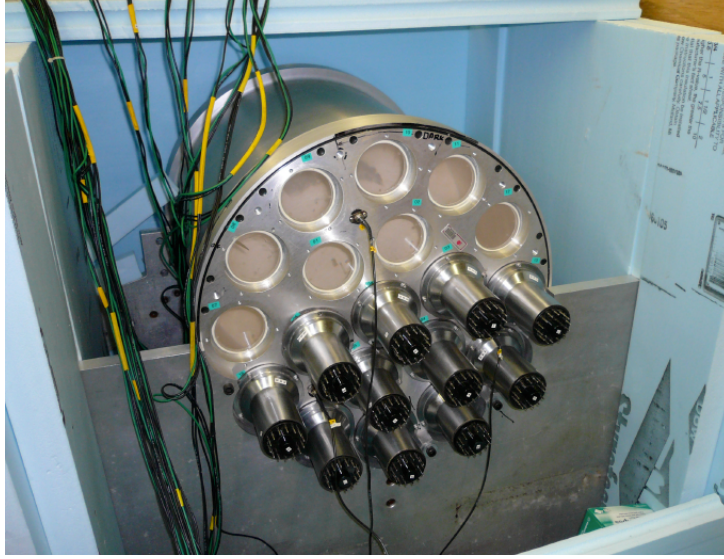
Figure 3.14: Picture of the NaI crystal from its backside [3].
