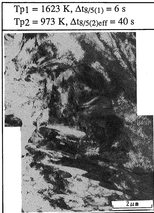
Fig. 11 TEM micrograph of the blocky structure
