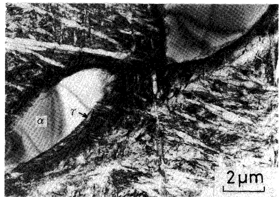
Fig. 11 Transmission electron micrograph for \alpha + \beta quenched Ti-6Al-4V alloy cathodically charged at 4200 A/m 2 for 14.4 ks.
