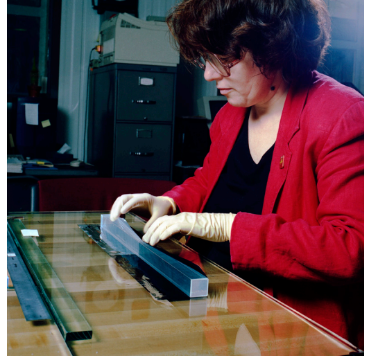
Figure 2.14: A CsI crystal being wrapped with an aluminized mylar. (Picture: Fermilab Visual Media Services)
