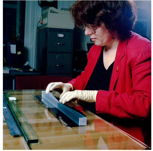
Figure 2.14: A CsI crystal being wrapped with an aluminumized mylar. (Picture: Fermilab Visual Media Services)
