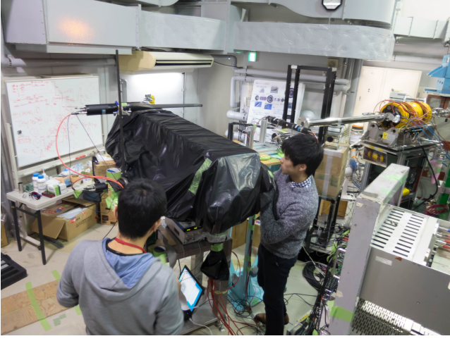
Figure 6.45: A photograph of the beam test apparatus. A small CsI calorimeter was installed inside the box covered by black sheets. Two plastic scintillator trigger counter were placed in front of the CsI calorimeter.
