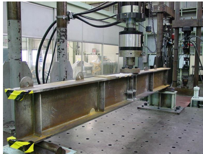
Fig.2.7 Test beam model under three point bending.
