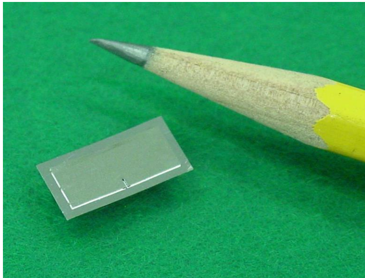
Fig.A.1 Fatigue Damage Sensor (FDS) with a pencil tip.
