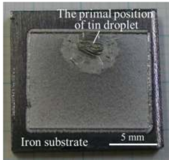
Fig. 4.8 Appearance of laser-irradiated surface of Fe substrate after wetting experiment with liquid Sn.
