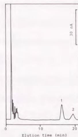
Fig. 31. Analysis of the reduced oligosaccharides derived from porcine erythrocyte ghost. Eluent: 0.5 M sodium hydroxide solution. Other conditions as in Fig. 25. Sample scale: 73 \mu l as blood. Peak assignment: 1 = [O-6], 2 = [O-7].
