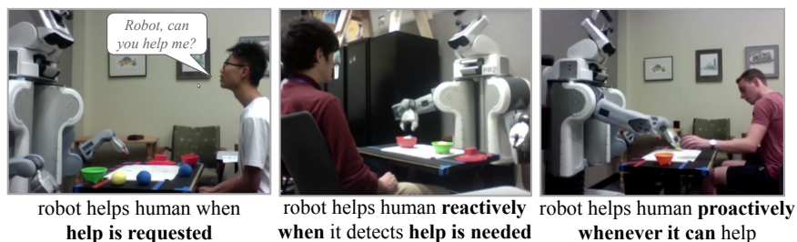
Figure 5.1: Different initiative models for robot assistance during collaborative task executions: human-initiated help (left), robot-initiated reactive help (middle), and robot-initiated proactive help (right).
