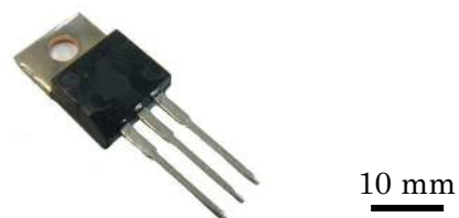
Fig. 6.11 SiC TO-220 package formed using CAZAC.
