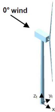
Figure 2.3 Tower-base co-ordinate system. (Reproduced from Reference [26])
