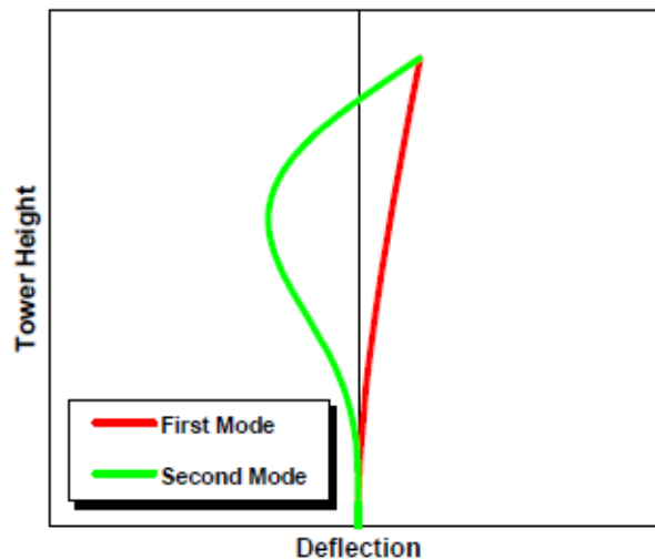
Figure 2.10 Tower mode shapes. (Reproduced from Reference [26])
