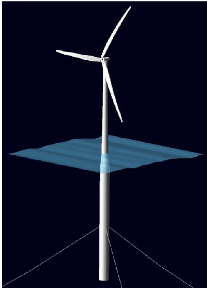
Figure 3.1 Illustration of the NREL 5-MW wind turbine on the OC3-Hywind spar. (Reproduced from Reference [44])
