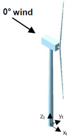
Figure 2.3 Tower-base co-ordinate system. (Reproduced from Reference [26])
